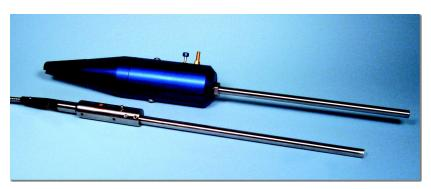
The Process RamanProbe combines the best features of optical design and mechanical robustness for laboratory and process monitoring. To protect the optics from extreme heat, the probe body is kept at a distance from the reactor with an extension tube. The tube itself can be interfaced directly into reactors and process lines. With the optional purgeable housing, the probe is suitable for most industrial environments.
