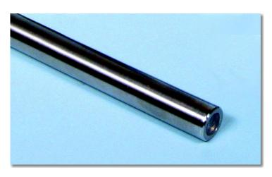
The RPR1064 is the only FT-Raman fiber optic probe that can be used at elevated temperatures and up to 1500 psi. It is comparable to our Reaction RamanProbe<sup>TM</sup> for dispersive Raman instruments. The outer sleeve is constructed with 316 stainless-steel with a sapphire window. For optimum resistance to corrosive chemicals, the probe sleeve is also available in Hastelloy C construction with a gold gasket.
