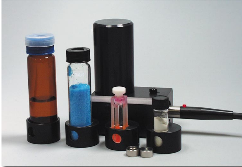
Compact sample holder with four inserts.
