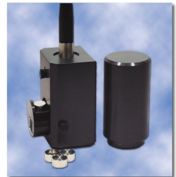
Solid sampling with the entire holder tipped on end.
