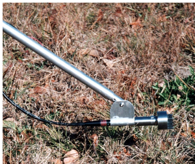
Figure 3. SERS vapor probe that incorporates a roughened gold substrate, fiber optic probe, and fan.
