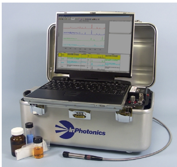
Figure 1. Typical identification result from the InPhotote™ portable Raman spectrometer. The HQI (hit quality index) is the distance from the unknown spectrum to the library result (i.e. lower HQI is a better match).
