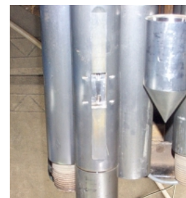
Above: A cone penetrometer truck (CPT) stabilized for cone deployment. Right: Cone tip and rod sections showing viewport for sensor implementation.
