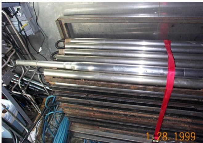
Inside the CPT: (Upper) The Raman spectrometer system, data station, and fiber optic cables. 1 (Lower) Cone rods with prestrung fiber cable await deployment.
