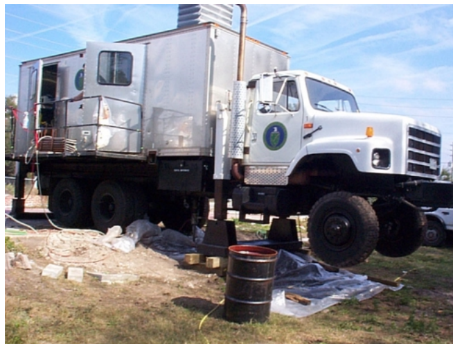
Above: A cone penetrometer truck (CPT) stabilized for cone deployment. Right: Cone tip and rod sections showing viewport for sensor implementation.
