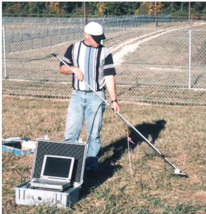
Detecting landmines in a test field using a portable spectrograph and SERS probe. 2
